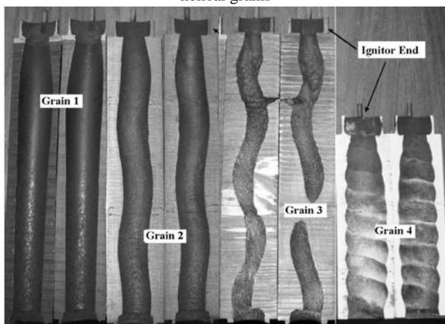
Figure 18 – Post-Test fuel grain cross sections
