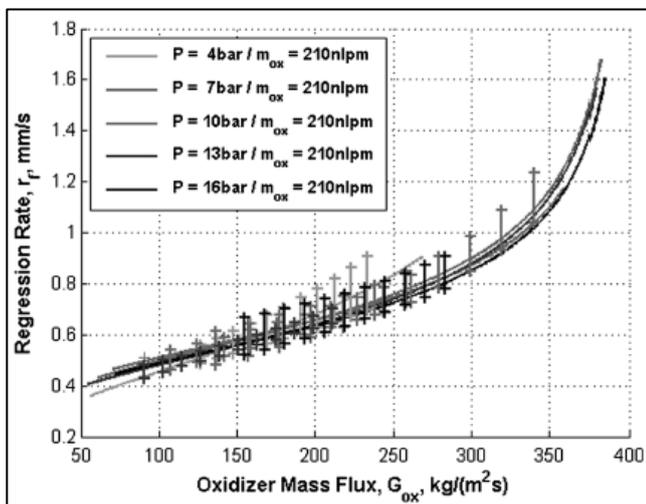
Figure 9 – Instantaneous ensemble regression rate showing negligible pressure dependence
