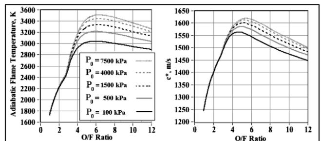
Figure 11 – Thermodynamic and transport properties of N<sub>2</sub>O/ABS combustion products
