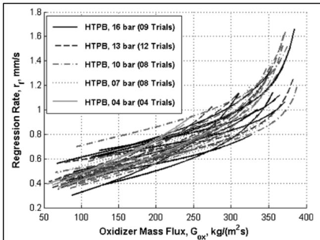
Figure 8 - Comparison of instantaneous regression rate for all the tests showing similar trends
