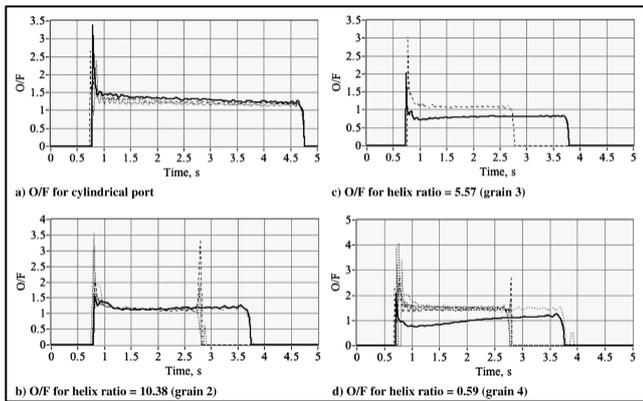
Figure 16 – GOX-ABS tests; Variation in O/F with burn time.
