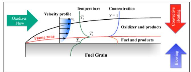
Figure 4 – Boundary Layer Combustion
