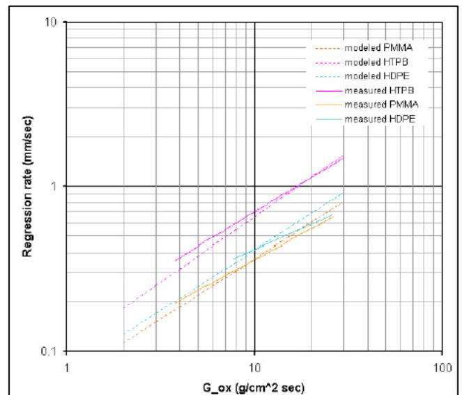
Figure 7 – Modeled average fuel regression rate with oxygen.
