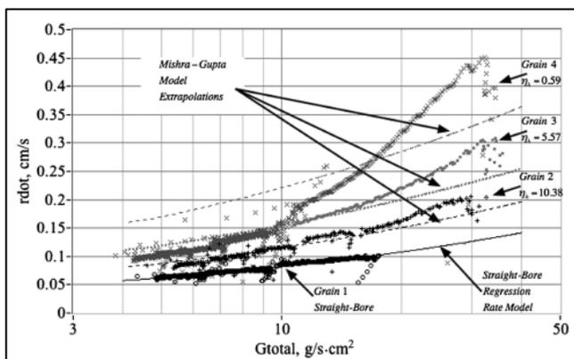
Figure 17 – GOX-ABS regression rate for straight-bore and helical grains
