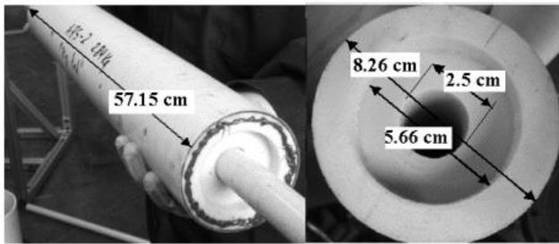
Figure 12 – ABS Fuel grain dimensions
