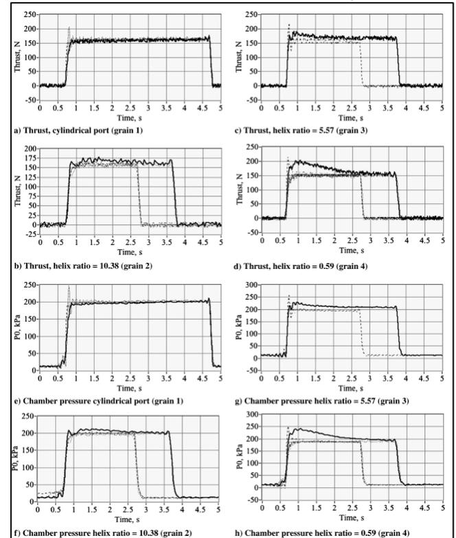
Figure 14 – GOX-ABS tests; Thrust and chamber pressure time histories
