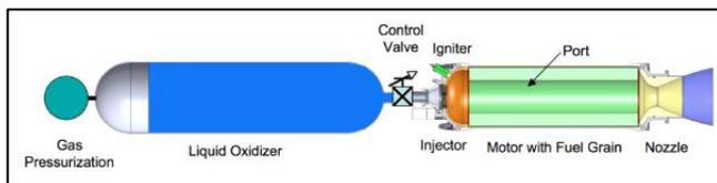
Figure 3 – Hybrid Rocket System
