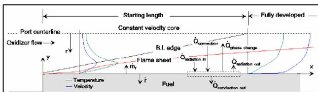
Figure 5 – Zilliac's Conceptualization of Flow and Energy Balance within hybrid rocket motor
