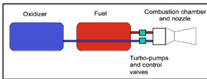
Figure 1 – Liquid Propellant Rocket System
