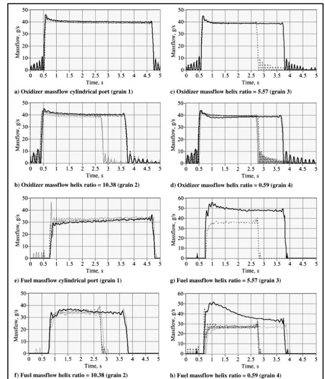
Figure 15 – GOX-ABS tests; Oxidizer, and fuel mass flow rate time histories.
