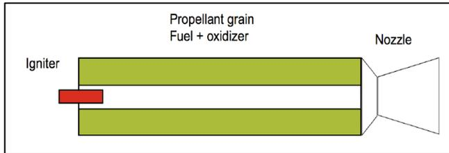
Figure 2 – Solid Propellant Rocket System
