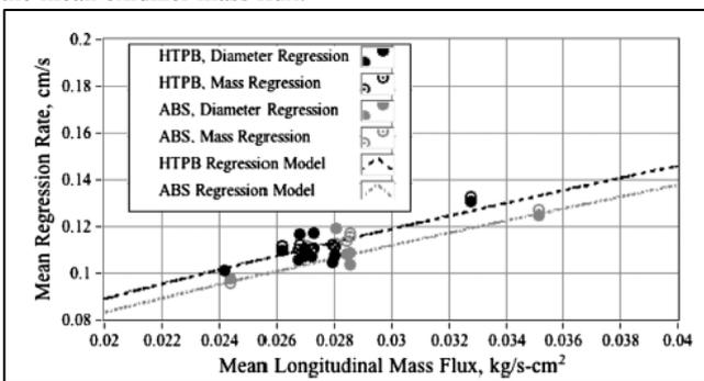
Figure 13 – Predicted and measured linear regression for HTPB and ABS fuel grains
