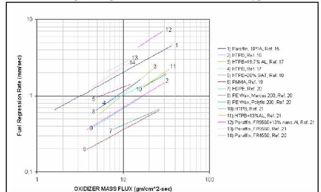
Figure 6 – Average fuel regression rate with oxygen
