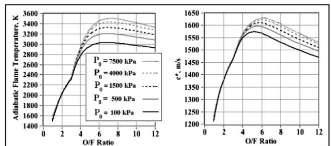
Figure 10 – Thermodynamic and transport properties of N<sub>2</sub>O/HTPB combustion products
