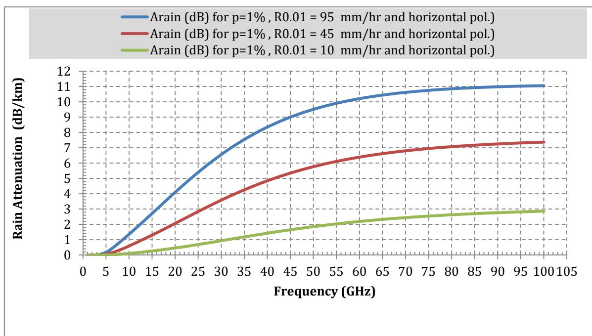
Figure 3 Rain (dB) attenuation for  $p = 0.01$  and the horizontal polarization for %  $R_{0.01\%} = 10 \text{ mm.hr}, 45 \text{ mm.hr}$  and  $95 \text{ mm.hr}$
