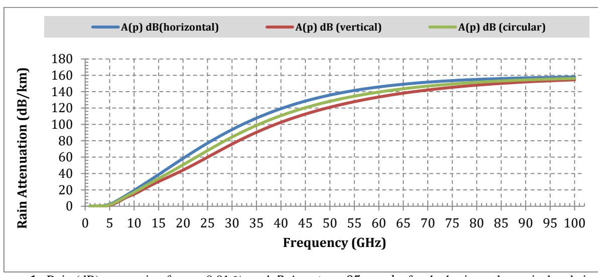
Figure 1 Rain (dB) attenuation for  $p=0.01\%$  and Rain rate = 95 mm.hr for the horizontal , vertical and circular polarization
