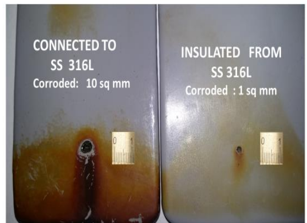
Fig. 3. Test panels after 14 days in North Sea water tank coupled ( left ) and insulated ( right ) from immersed SS 316 L details.
