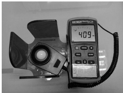
Fig. 5. Light penetration is measured by using a light meter (Model: EXTECH instrument EasyView™ 30 light meter).
