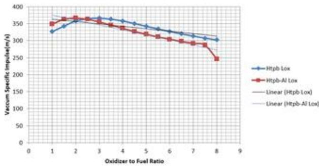
Fig. 7 HTPB-Lox, with and without additive
