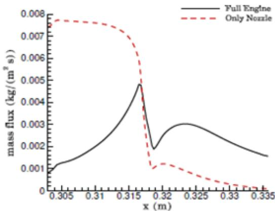
Fig. 16 Mass flux distribution due to wall ablation
