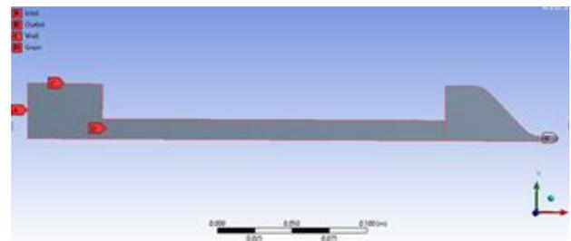
Fig. 11 Preliminary design with the wall, inlet, outlet, and grain
