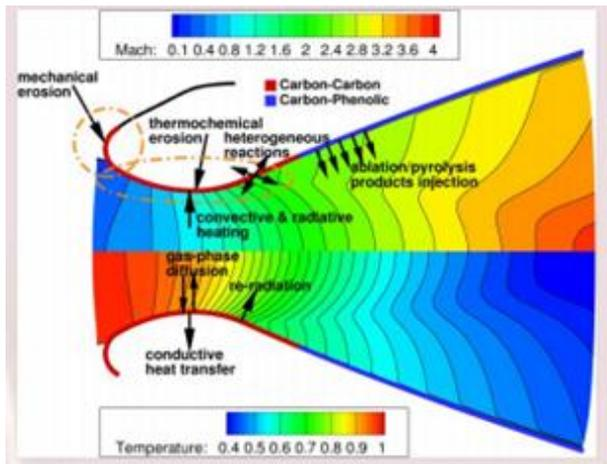
Fig. 14 An illustration of the erosion process in a nozzle
