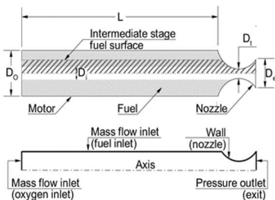
Fig. 3. Illustration of a hybrid rocket engine
