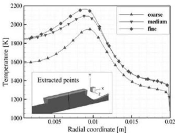
Fig 13 Variations in temperature with the mesh types
