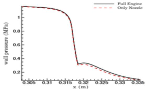
Fig 18 Pressure distribution due to wall ablation
