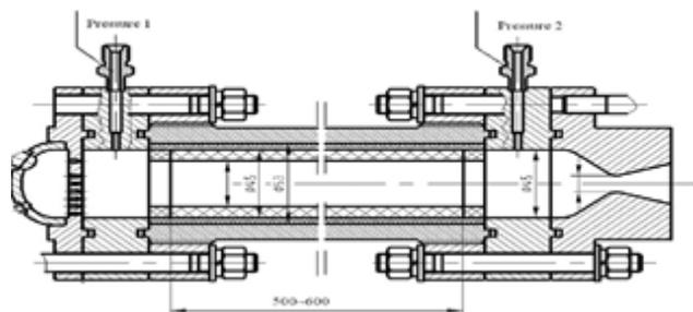
Fig. 9 Hybrid rocket motor for an experimental test
