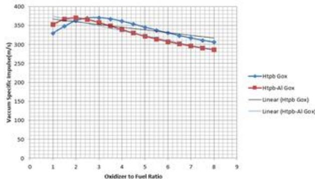
Fig. 8 HTPB-Gox, with and without additive
