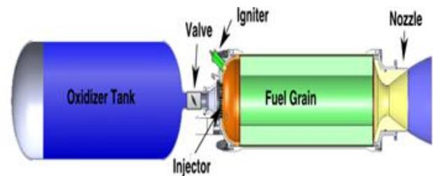
Fig. 2 Engine principle
