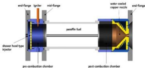
Fig. 4. An example of the application of Paraffin fuel with Aluminum additive, experimental setup
