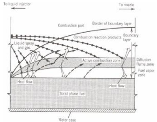
Fig. 10 Flow complexity in a hybrid rocket combustion chamber
