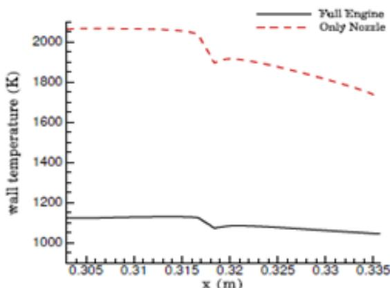
Fig. 17 Temperature distribution due to wall ablation
