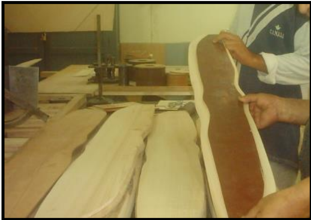
Fig. (7) Cutting the prop blank to size
