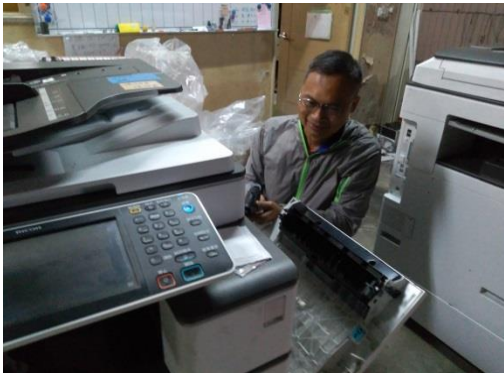
Fig.5 The inspection of the fusing system
