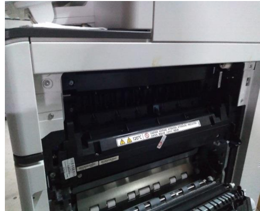
Fig.7 The fusing system that has been inspected
