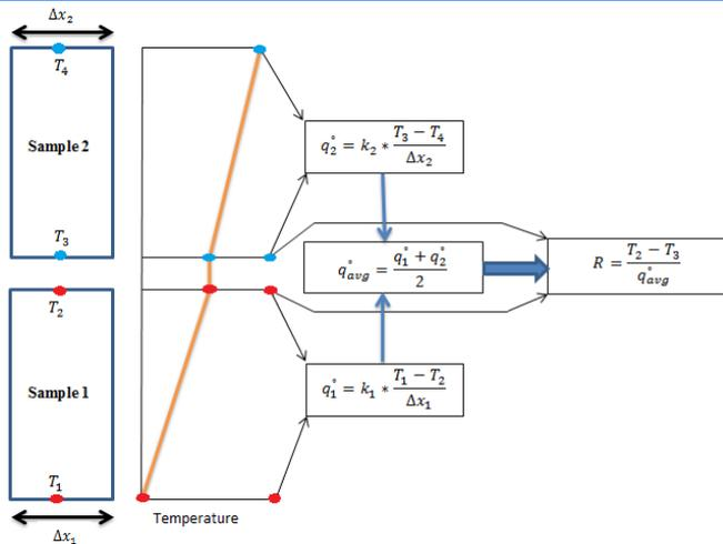
Fig. (3) Graphical representation of calculation procedure
