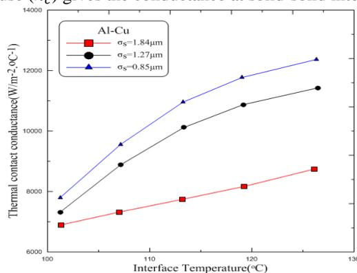
Fig. (5) Effect of interface temperature on TCC
