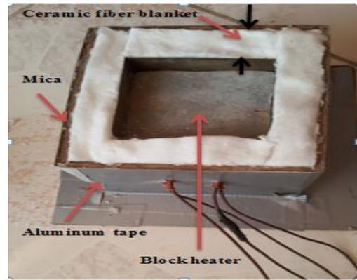
Fig. (2) Insulation layers of block heater
