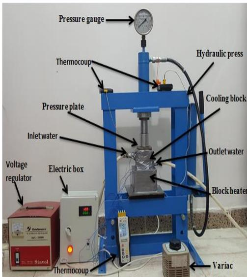
Fig. (1) Photography view of the test rig with instruments and measurements devices
