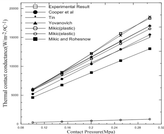
Figure (6) Comparison between experimental results with models
