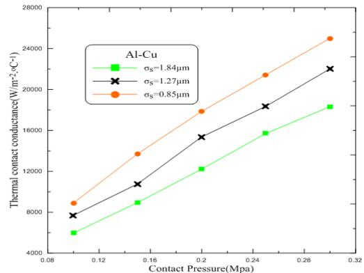
Fig. (4) Effect of contact pressure on TCC
