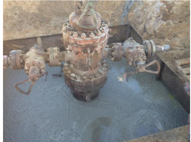
Figure 6: Wellhead with pumped slurry cement to avoid the smell gas
