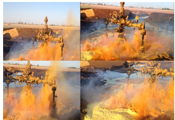
Figure1: Wellhead with blowout statement
