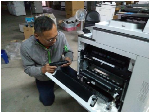
Fig.6 The inspection of the duplex system
