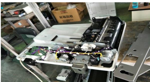
Fig.7 The toner cartridge and the toner roller system after inspecting and repairing
