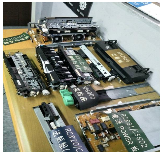
Fig.14 The toner cartridge, power distribution board, paper feed tray, paper output tray have been repaired and tested
