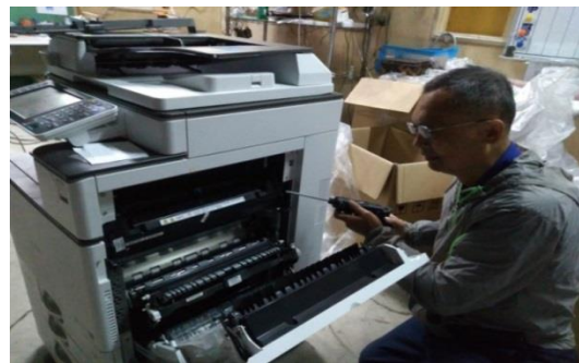
Fig.13 The troubleshooting of the paper supply group
