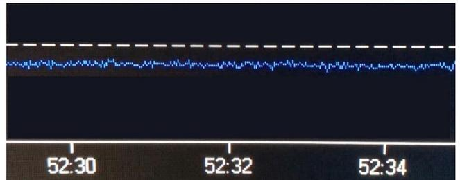
Fig. 10: Graphic of the z-axis gravity acceleration measured by the accelerometer when it is aligned with the piezoelectric disc and the disc is reversely polarized, in the case of 4 glass acoustic barriers.
