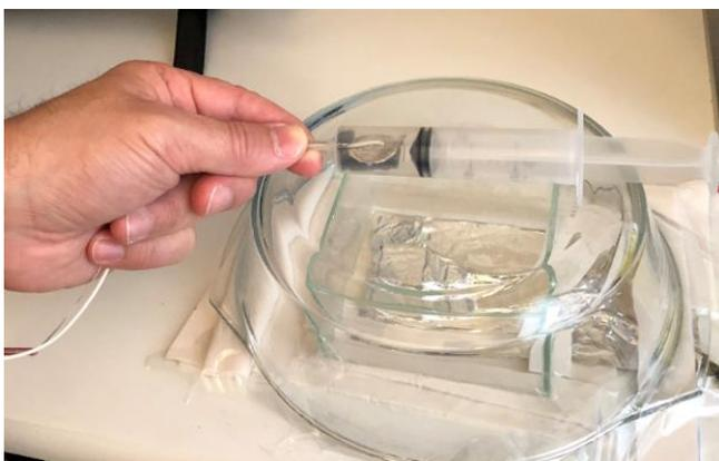
FIG. 4. Photo of the experimental setup established to detect the forces at distance. The piezoelectric disc was enclosed in the partial camera of the syringe. The distance between the z-sensor of the accelerometer and the disc was 10cm and the former was electromagnetically shielded with an aluminum foil and from external noises due to the two glass containers.
