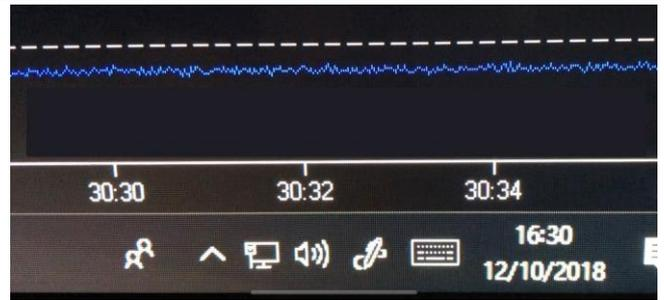
FIG. 2. Frame of the z-axis acceleration variation (vertical axis in  $m/s^2$ ) in 4s periods (horizontal axis in seconds) for the loudspeaker polarized in opposite mode in "on" period. The quantity of peaks is 56.
