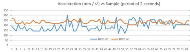
FIG. 6. Plot of the z-axis gravity acceleration variation (in  $\text{mm/s}^2$ ) of the setup with 10cm distance between emitter and accelerometer versus samples of measurement of 2s periods. The two curves represent the period "on" and period "off" in order to make comparison.
