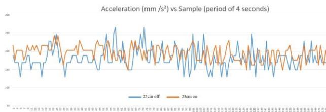
FIG. 9. Plot of the acceleration variation (in mm/s<sup>2</sup>) of the setup with distance 25 cm versus samples of measurements for 4s periods. Two curves (period "on" and period "off") are shown for comparison.
