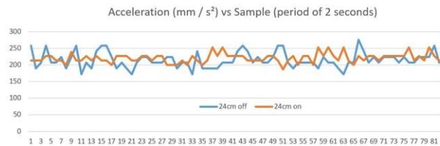
FIG. 8. Plot of the acceleration variation (in mm/s<sup>2</sup>) of the setup with distance 24 cm versus samples of measurements (in s) for two curves (period "on" and period "off"), in order to make comparison.
