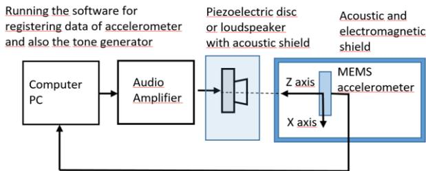
FIG. 1. Scheme of the basic experimental setup of the experiments performed in order to detect forces at distance by the piezoelectric device or the loudspeaker. In the right side, it is indicated the accelerometer used in the measurements which is connected to the computer for collecting all the acceleration data.
