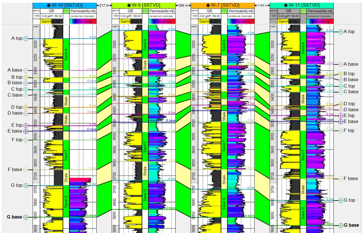
Figure 8: Permeability log estimated in K-field using well logs
