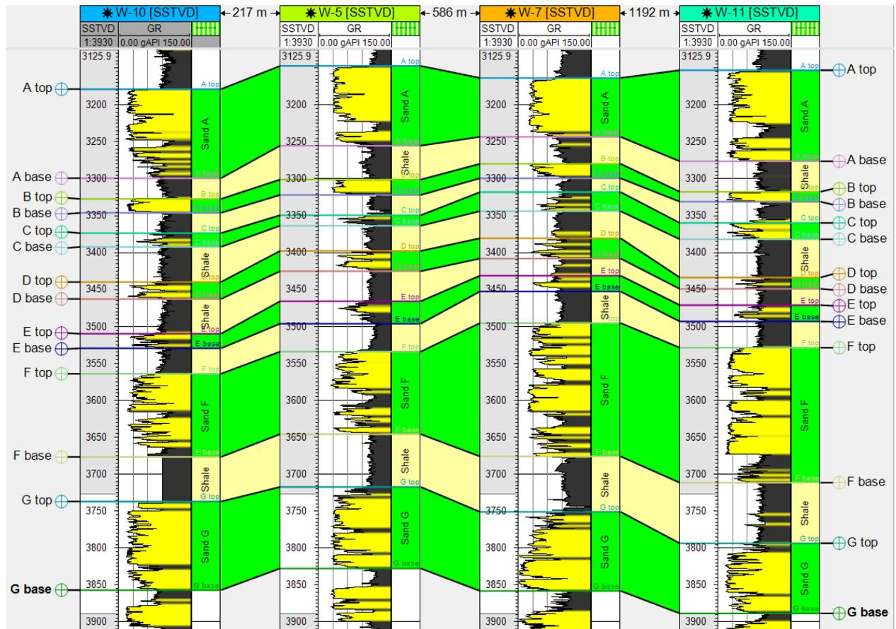
Figure 3: Lithofacies identified in K-field using well logs
