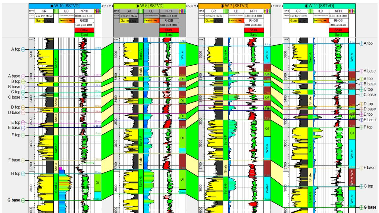
Figure 6: Fluid types estimated in K-field using well logs
