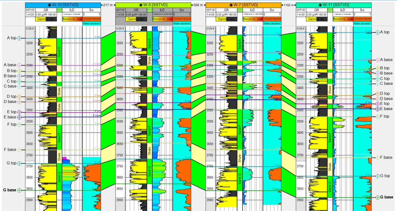
Figure 7: Fluid saturation logs estimated in K-field using well logs
