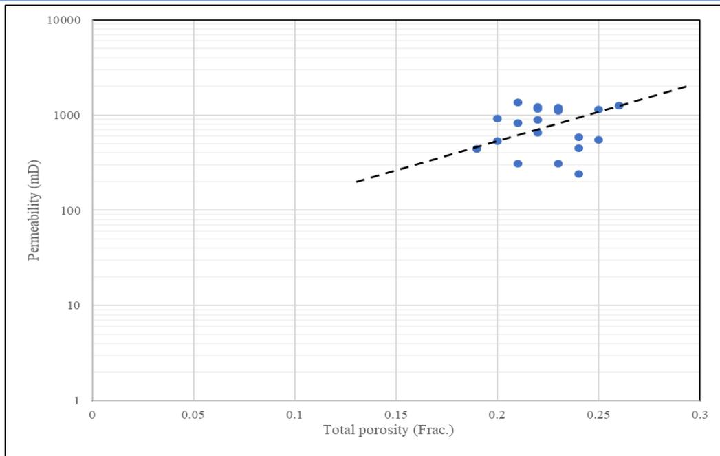
Figure 13: Cross-plot of porosity versus permeability for reservoirs in K-field
