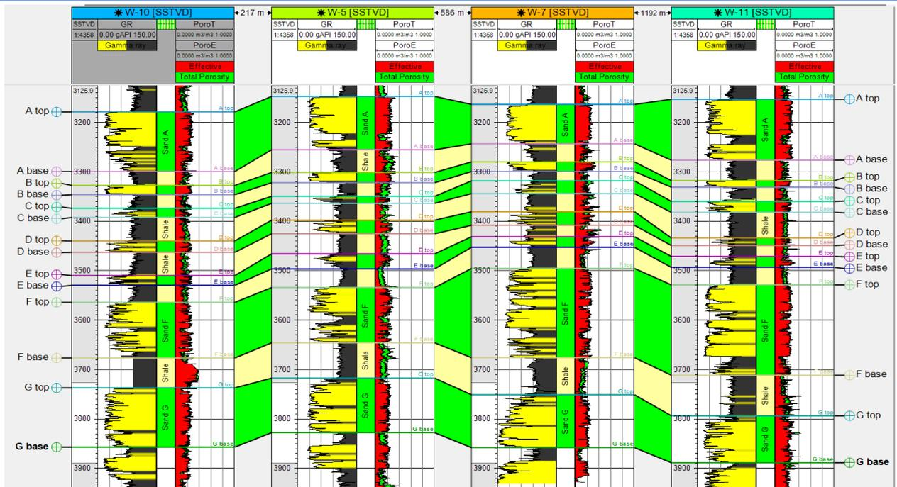
Figure 5: Total and effective porosity logs estimated in K-field using well logs
