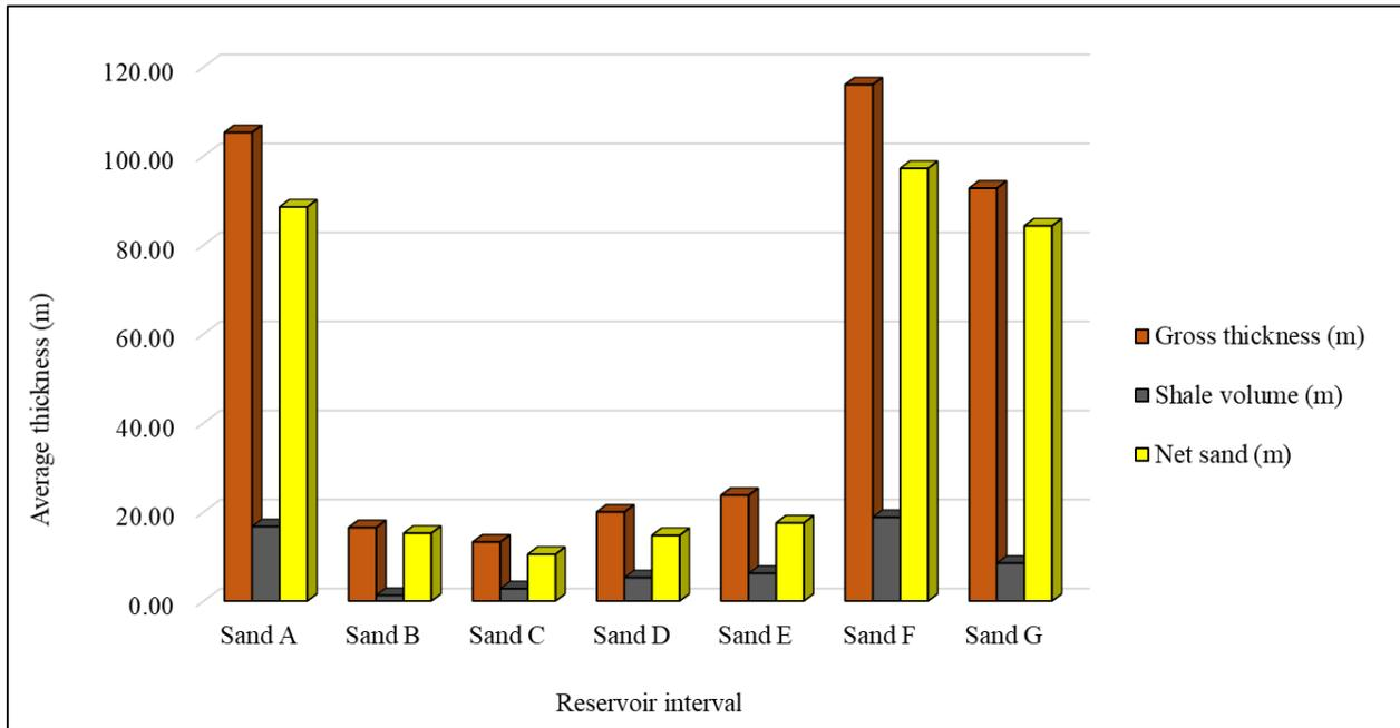
Figure 9: Average gross thickness, shale volume and net sand thickness across the field
