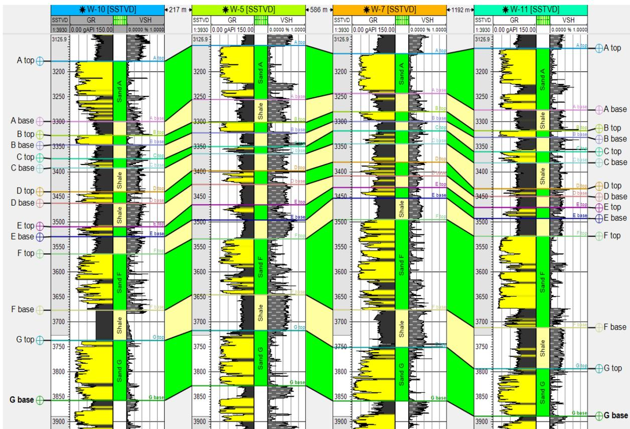
Figure 4: Shale volume log estimated in K-field using well logs
