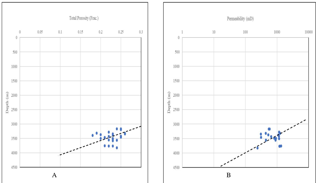
Figure 12: (A) Cross-plot of porosity versus depth for reservoirs in K-field. (B) Cross-plot of permeability versus depth for reservoirs in K-field.
