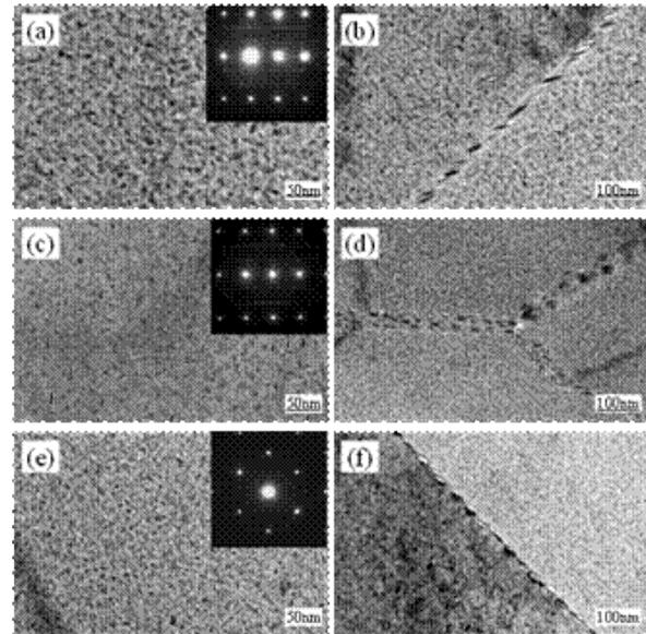
Figure 5 TEM images of the precipitates in grain interiors and grain boundaries for 7056 Al alloys after various heating aging rates: (a) (b) 20°C/h; (c) (d) 40°C/h; (e) (f) 60°C/h.
