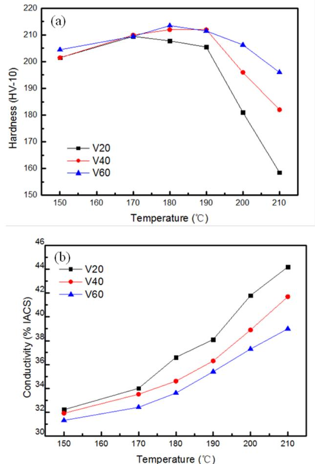
Figure 1 Effects of heating rate on (a) hardness and (b) electrical conductivity of 7056 Al alloys.
