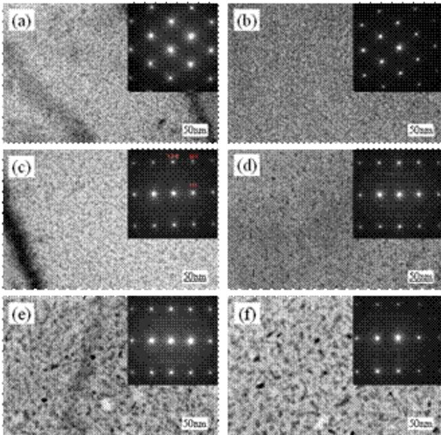
Figure 6 TEM bright-field images of the grain precipitates of 7056 Al alloy aged at various ending temperatures at a heating rate of 40 °C/h: (a) 150 °C; (b) 170 °C; (c) 180 °C; (d) 190 °C; (e) 200 °C; (f) 210 °C.
