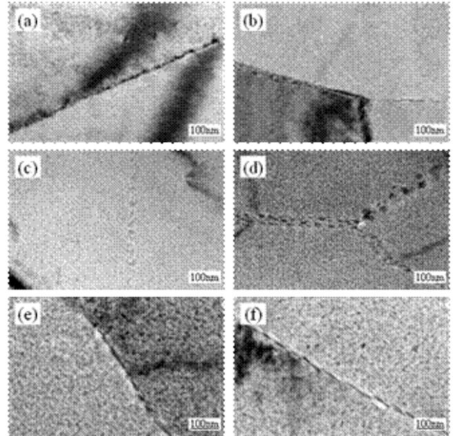
Figure 7 TEM bright-field images of the precipitates on grain boundaries of 7056 Al alloy aged at various ending temperatures at a heating rate of 40 °C/h: (a) 150 °C; (b) 170 °C; (c) 180 °C; (d) 190 °C; (e) 200 °C; (f) 210 °C.
