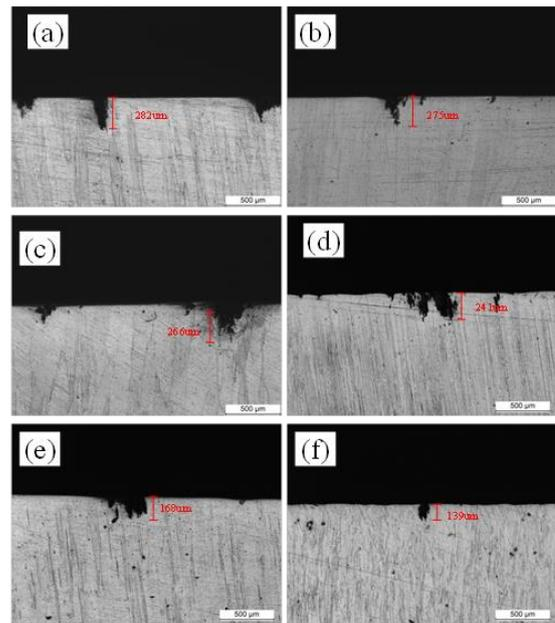
Figure 3 Cross-section corrosion morphologies and maximum corrosion depths of 7056 Al alloys aged at various ending aging temperatures at a heating rate of 40 °C/h: (a) 150 °C; (b) 170 °C; (c) 180 °C; (d) 190 °C; (e) 200 °C; (f) 210 °C.
