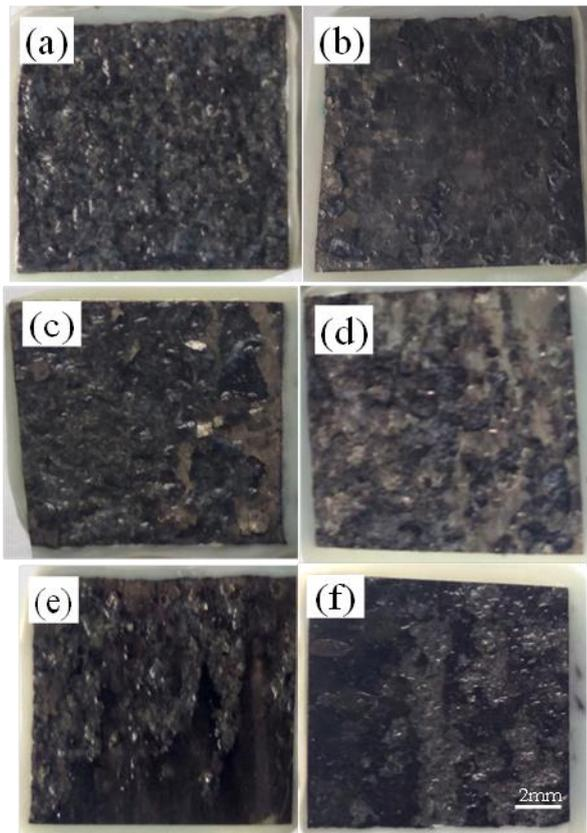
Figure 4 Surface morphologies of 7056 Al alloys after immersion in the EXCO solution for 48 h: (a) 150 °C; (b) 170 °C; (c) 180 °C; (d) 190 °C; (e) 200 °C; (f) 210 °C.
