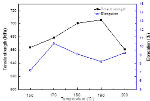
Figure 2 Variation of the ultimate tensile strength and elongation of 7056 Al alloy subjected to non-isothermal aging at a heating rate of 40 °C/h.
