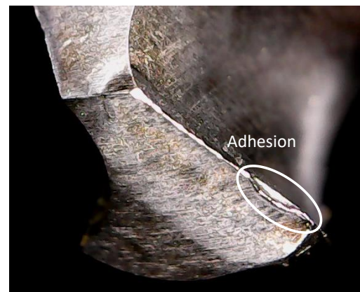
Fig. 9. Adhesive and flank wear observed in the uncoated commercial drill – CWD.
