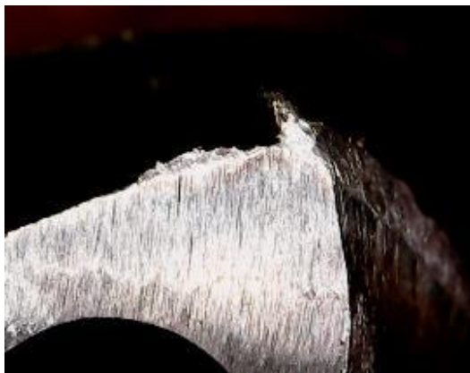
Fig. 7. Chipping of the cutting edge in the nitrided drill at 500 °C – N500.
