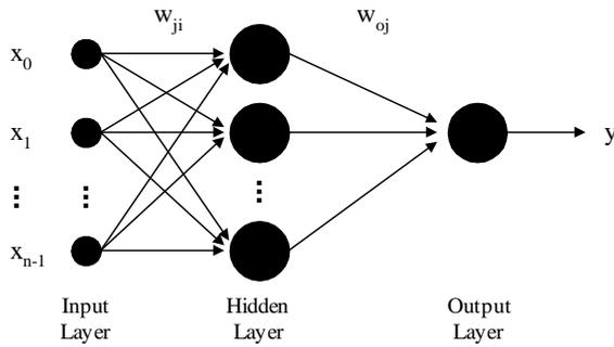
Fig. 2: Multilayer Perceptron Neural Network with one hidden layer [12]
