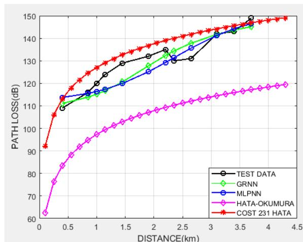
Fig. 6: Model Comparison for BTS 4
