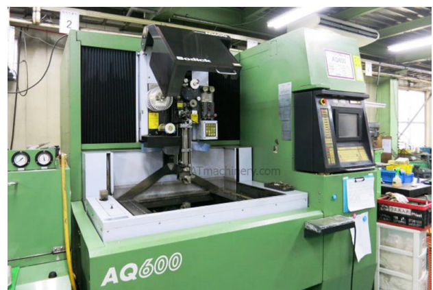
Fig 1. Sodick AQ600 electric discharge machining machine
