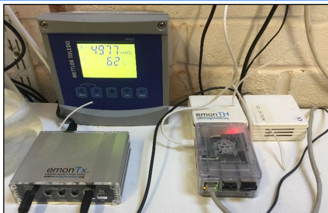
Fig. 2. EmonTX (front left), EmonHub (front right), Dissolved Oxygen Sensor (rear left), 2x EmonTH (rear right)
