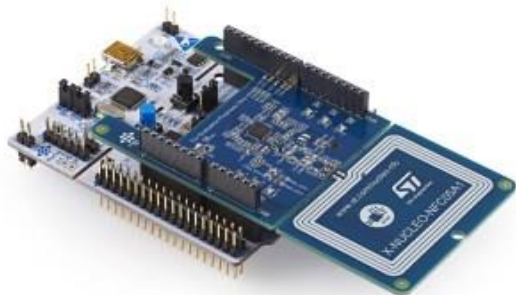
Fig. 4: The NFC development board (X-NUCLEO-NFC05A1 on top of an STM8 Nucleo board) based on ST25R3914 NFC reader [3]
