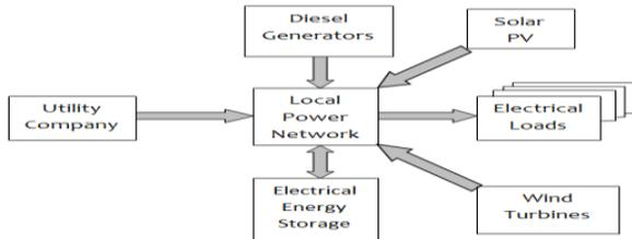
**Figure 1: The Distributed Energy Resources (DER) components in the case study onshore microgrid system**
