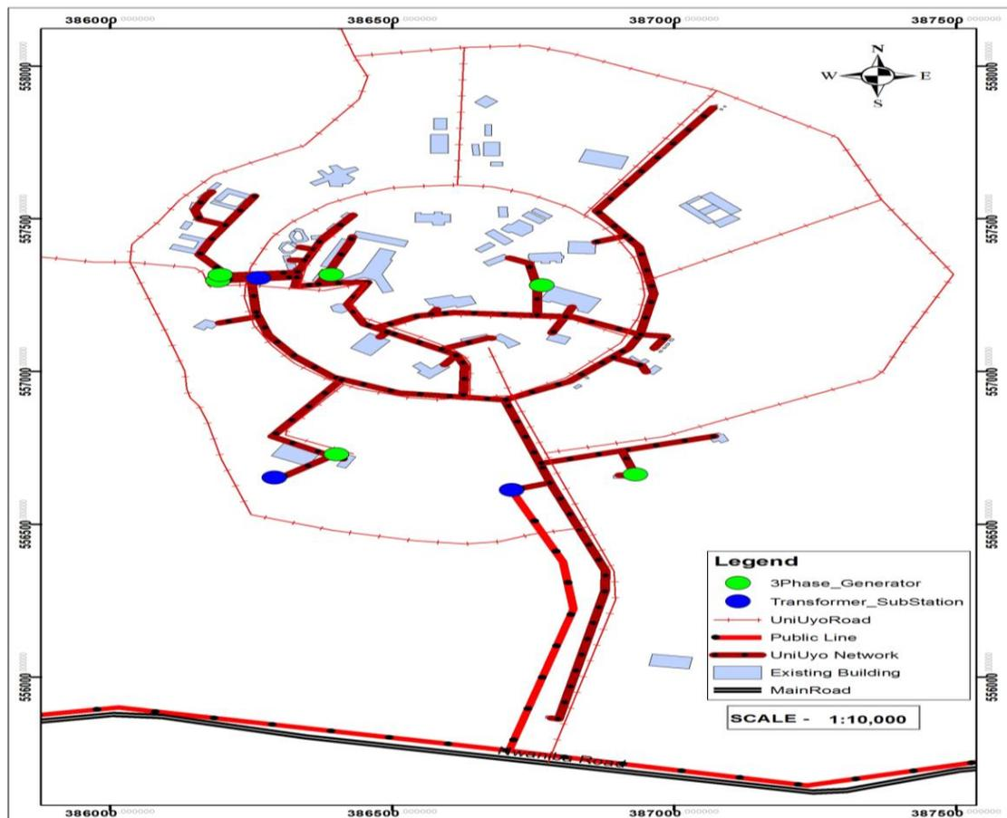
**Figure 2: University of Uyo Existing Electric Power Network**
