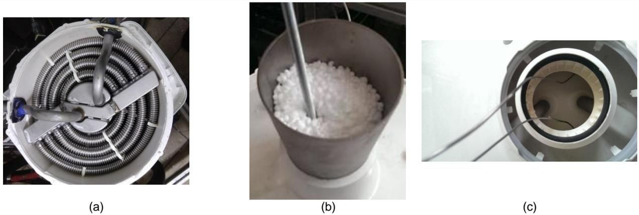
Fig. 1. Thermal battery
