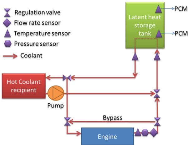
Fig. 9. Schematic presentation of the thermal battery on the engine test bench
