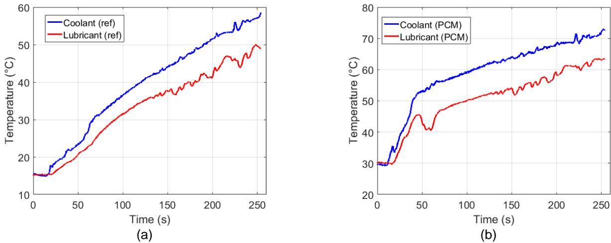
Fig. 12. Temperature profile on HDC without (a) and with (b) PCM
