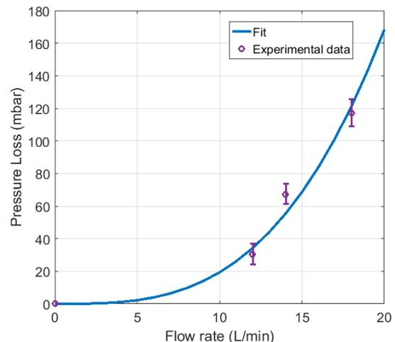
Fig. 5. Pressure drop of the storage tank
