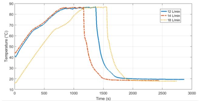
Fig. 3. PCM temperature behavior
