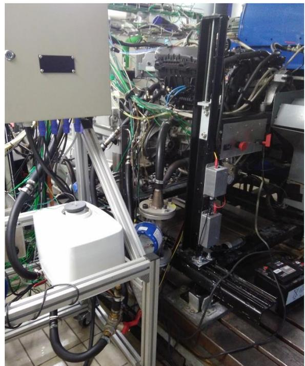
Fig. 8. The thermal battery installed on the engine test bench
