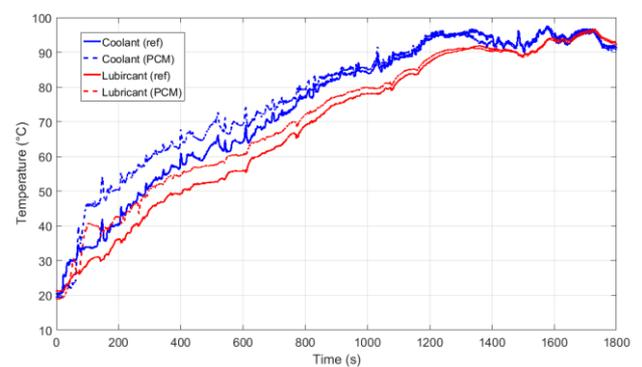
Fig. 11. Temperature profile evolution during WLTC with and without PMC
