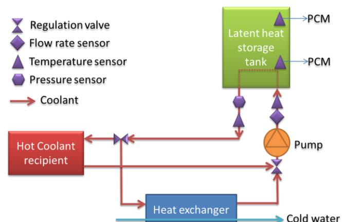
Fig. 2. Schematic presentation of the experimental setup
