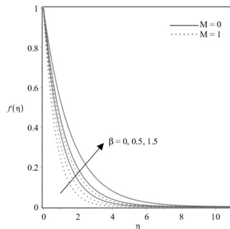
Fig. 1. Plots of velocity field for Deborah number and magnetic field parameter.
