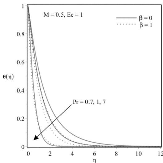
Fig. 4. Plots of temperature field for Prandtl number and Deborah number.
