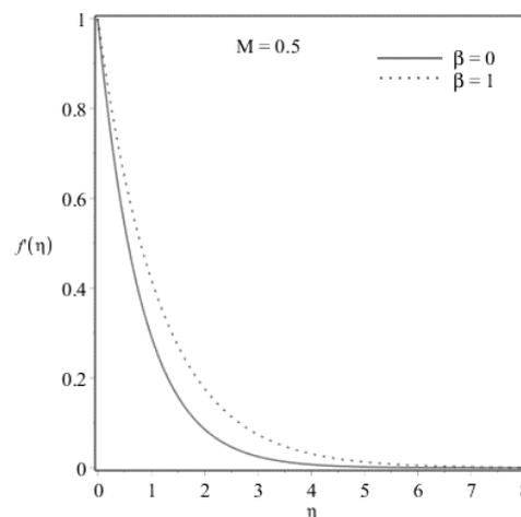
Fig. 2. Plots of velocity field for Deborah number and constant magnetic field parameter  $M$ .
