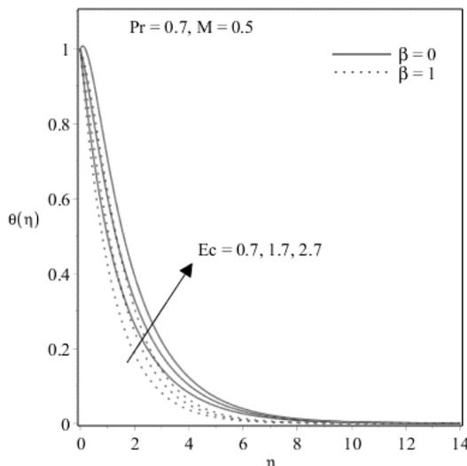
Fig. 5. Plots of temperature field for Eckert number and Deborah number.
