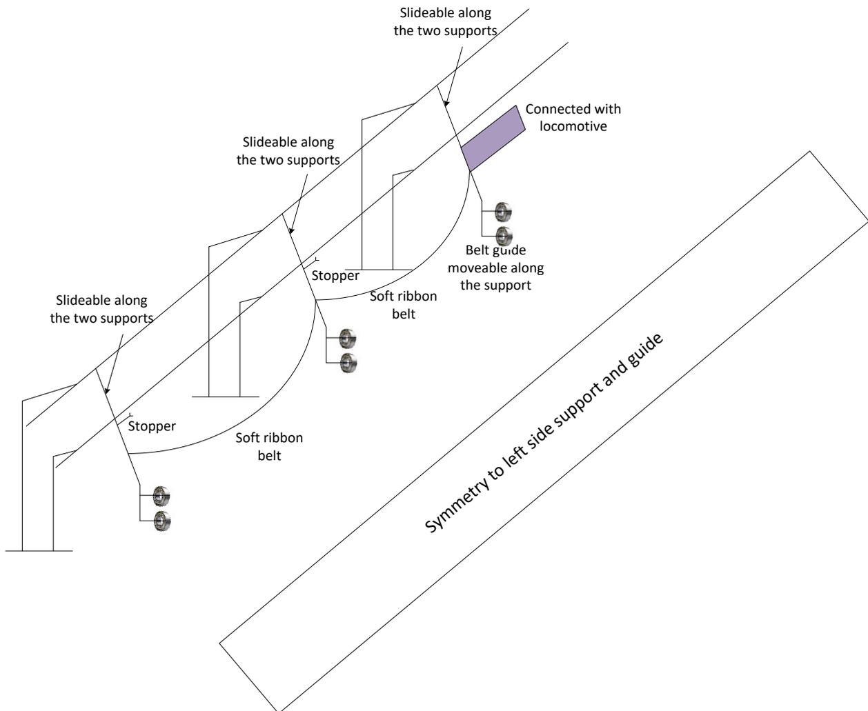
Fig. 7. Configuration 1 of horizontal guides for belt
