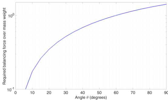
Fig. 2. Ratio of the levitation force to weight of the uplifted system versus angle  $\theta$
