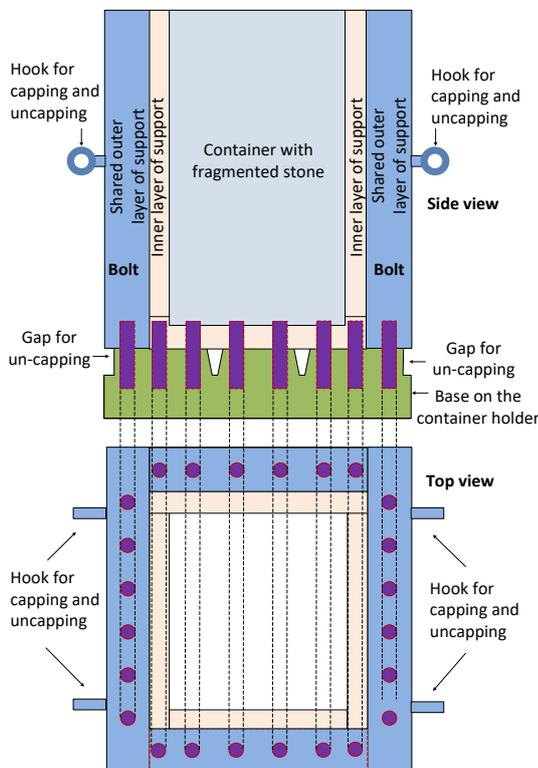
Fig. 10. Containers sitting on the container holder or base as shown in Fig. 6
