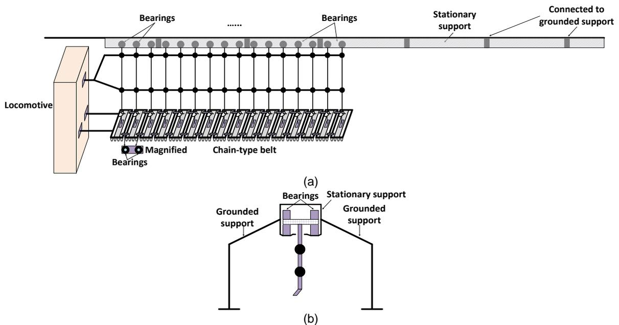
Fig. 8. Configuration 2 of horizontal guides for belt
