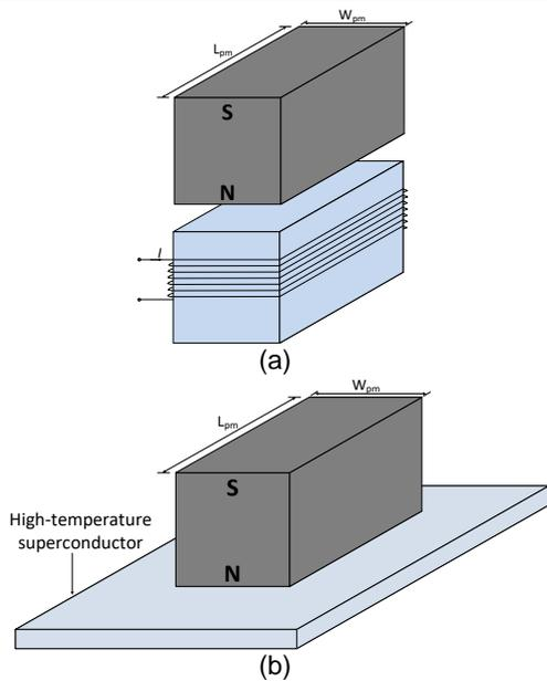
Fig. 9. Simplified model for magnetic levitation force calculation
