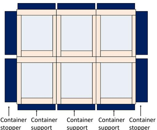
Fig. 11. Parked containers with heavy mass supported by the side support and back/front stopper
