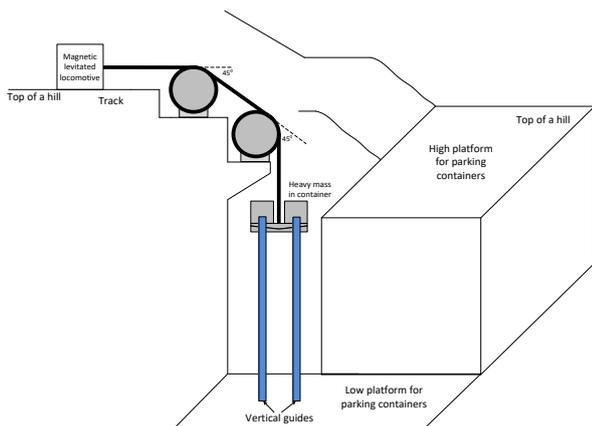
Fig. 3. Overall system with two wheels
