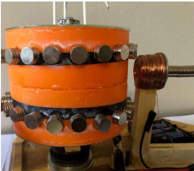
Photo 4: Side view of the device. Middle zone of V-format of magnets on drum
