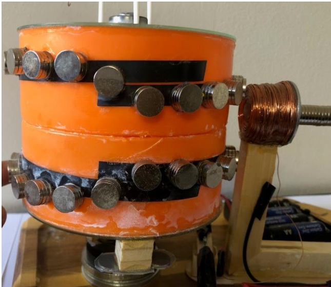
Photo 3: Side view of the device. Starting of V-format of magnets on drum
