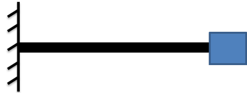
Figure 1. Schematic of the micro-beam with attached mass
