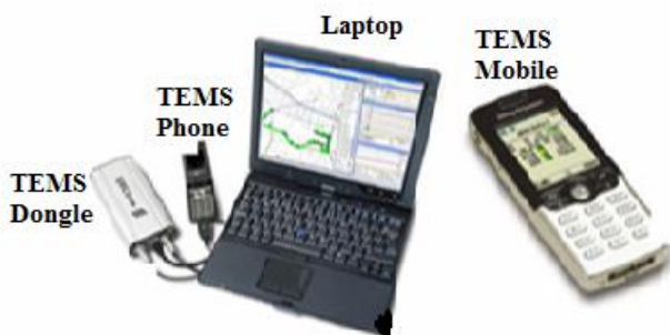
Fig. 1. Drive test measurement set.
