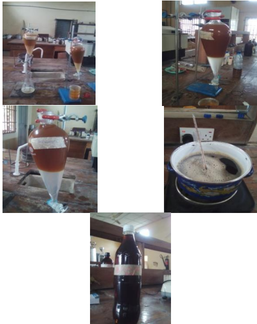
Stages 1 – 3; Washing of Biodiesel, Stage 4; Drying of biodiesel, Stage 5; final product. Figure 3: Washing and Drying of Biodiesel
