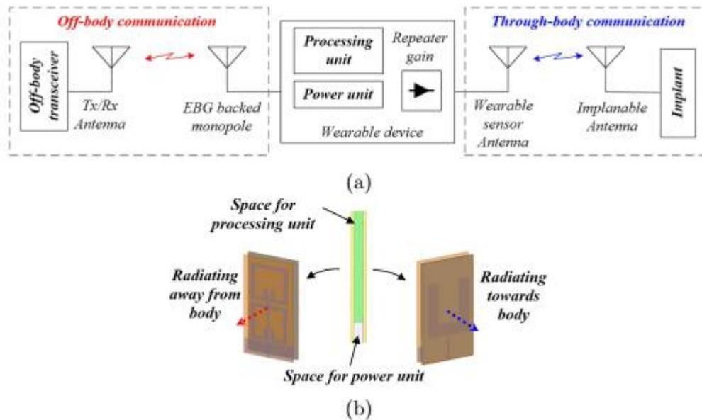
Fig. 4: (a) System level block diagram of implantable to outside-body transceiver connectivity via wearable node (b) Wearable device architecture representing the operational principle when two antennas radiate in the opposite directions.
