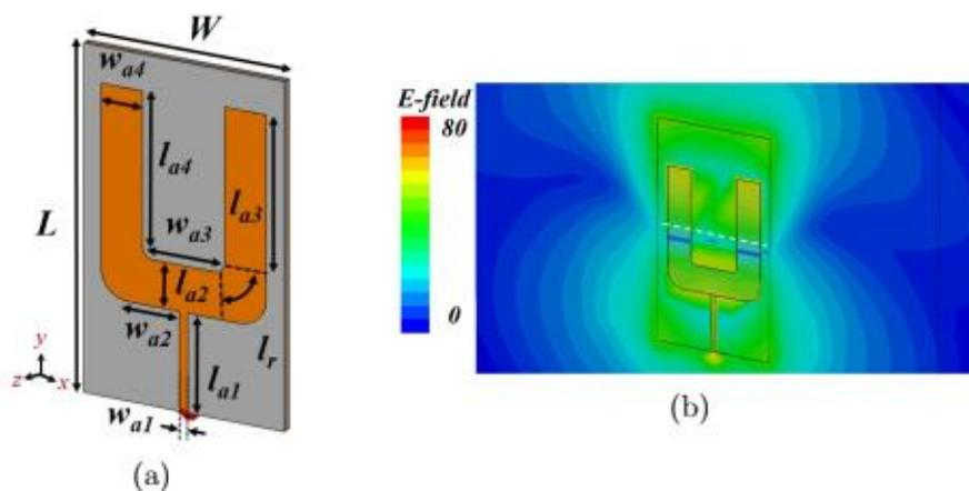
Fig. 1: (a) Diagrammatic of a wearable sensor antenna while  $L = 70$ ,  $W = 38$ ,  $w_{a1} = 2.05$ ,  $w_{a2} = 10.25$ ,  $w_{a3} = 7.33$ ,  $w_{a4} = 8.34$ ,  $l_{a1} = 22.60$ ,  $l_{a2} = 10.50$ ,  $l_{a3} = l_{a4} = 32.89$  (all measurements are in mm) (b) Normalized  $E$ -field arrangements.
