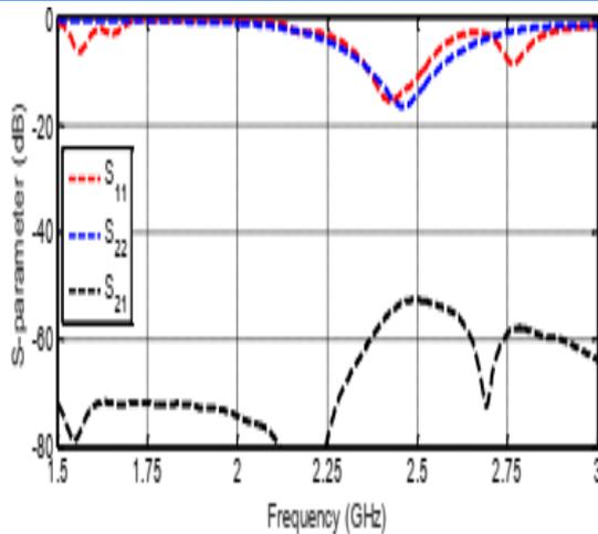
Fig. 7: Small frequency shift, which disturbs the impedance bandwidth of both the antennas, the simulated  $S_{11}$  and  $S_{22}$  remained below -10 dB at 2.45 GHz ISM band
