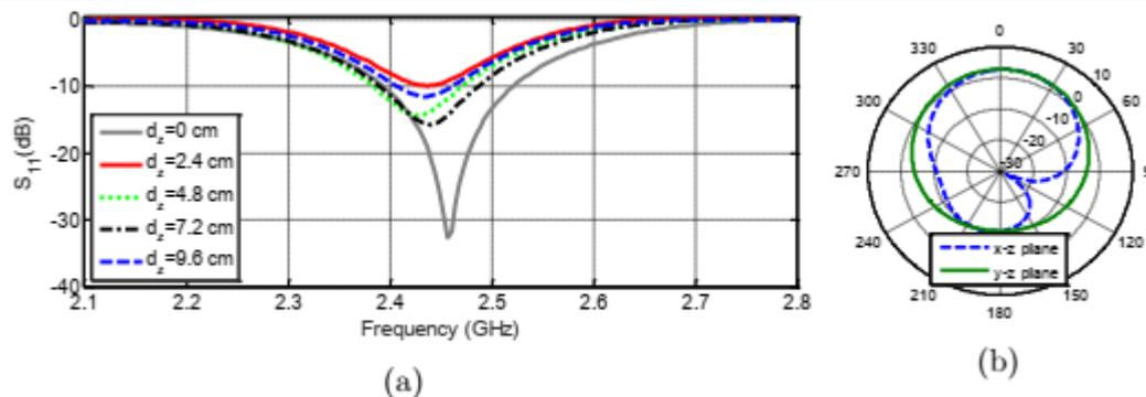
Fig. 3: (a) Simulated  $S_{21}$  when the antenna is placed on the chest and moved away from the body. (b) 2D gain plot
