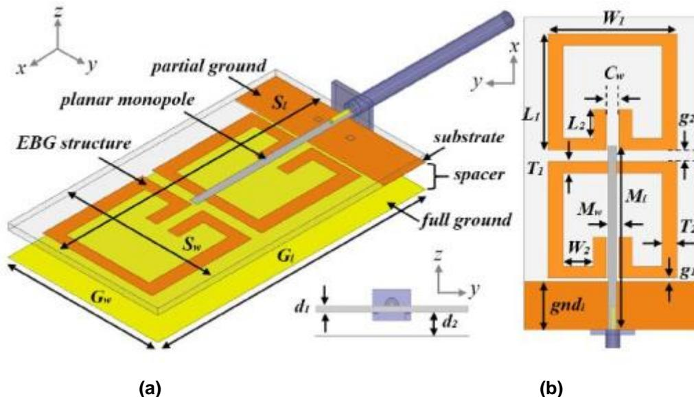
Fig. 2: (a) Configuration of the 2x1 EBG-backed planar monopole antenna with full ground (b) Top view of the monopole and finite sized EBG layer. The antenna is fabricated on semi-flexible Rogers RT/duroid 5880 substrates with  $\epsilon_r = 2.2$  and  $\tan\delta = 0.0009$ . © 2016 IEEE.
