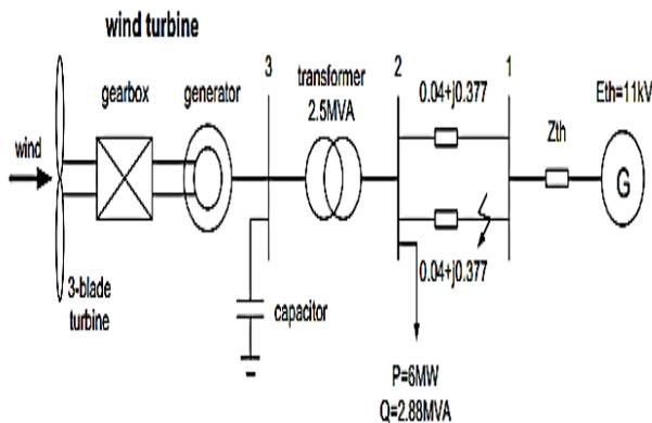
Fig. 4. Block diagram of a wind turbine connected to a grid
