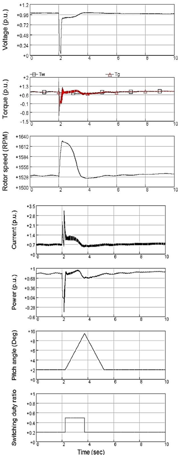
Fig. 9. Voltage, torque, generator rotor speed, current, output power, pitch angle and switching duty ratio in the case of combined control.
