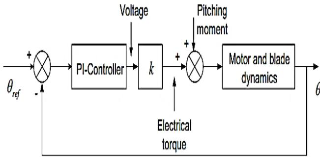
Fig. 3. Closed-loop pitch control mechanism.
