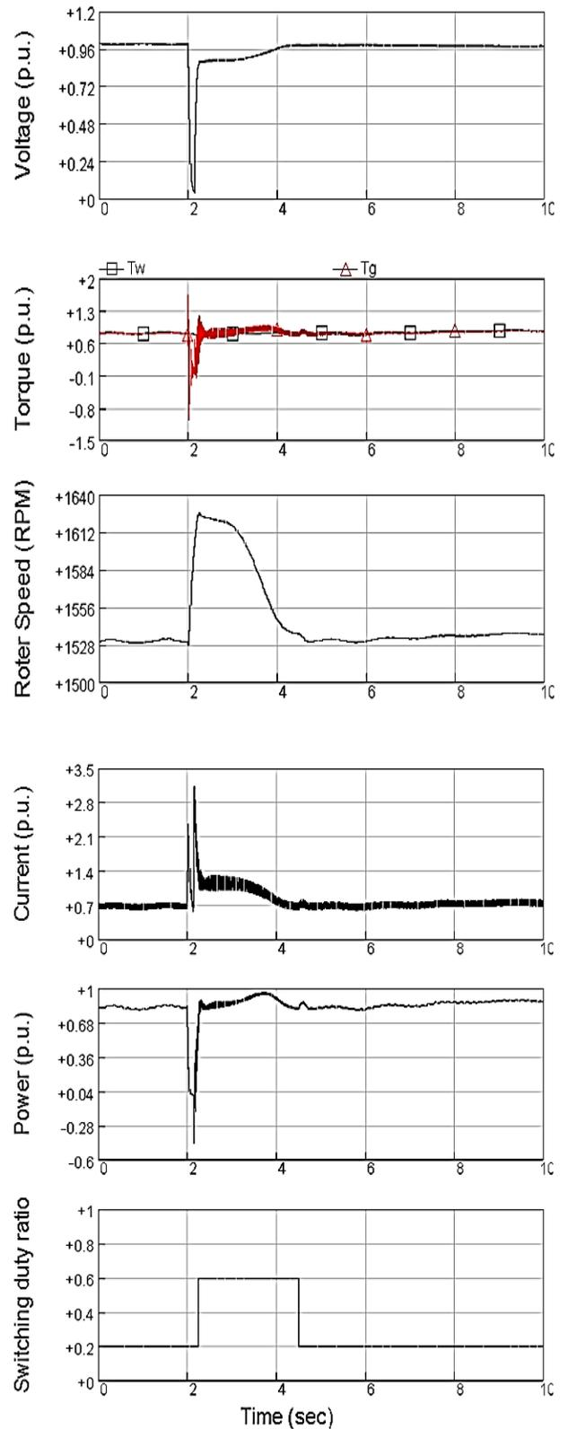
Fig. 8. Voltage, torque, generator rotor speed, current, output power and switching duty ratio in the case of dynamic slip control.
