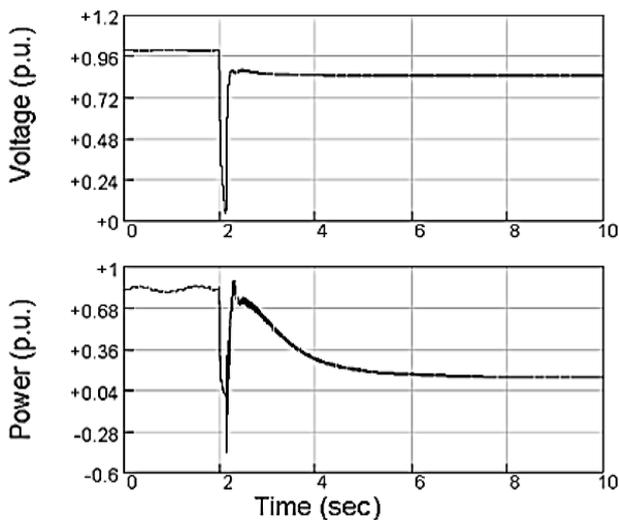
Fig. 6. Voltage and output power of the wind turbine in the case of unstable situation.
