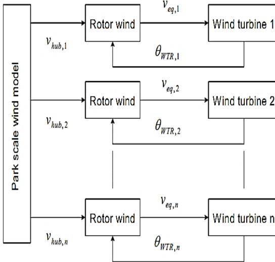
Fig.1. Structure of the wind model.
