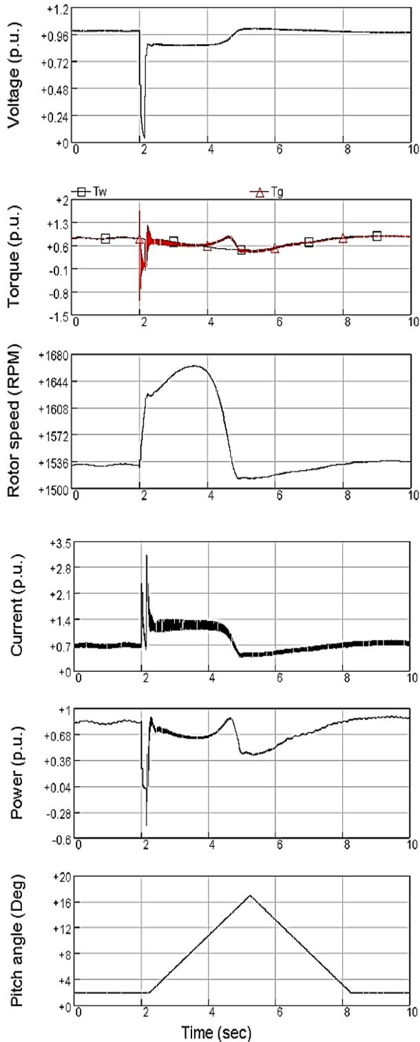
Fig. 7. Voltage, torque, generator rotor speed, current, output power and pitch angle in the case of pitch control.
