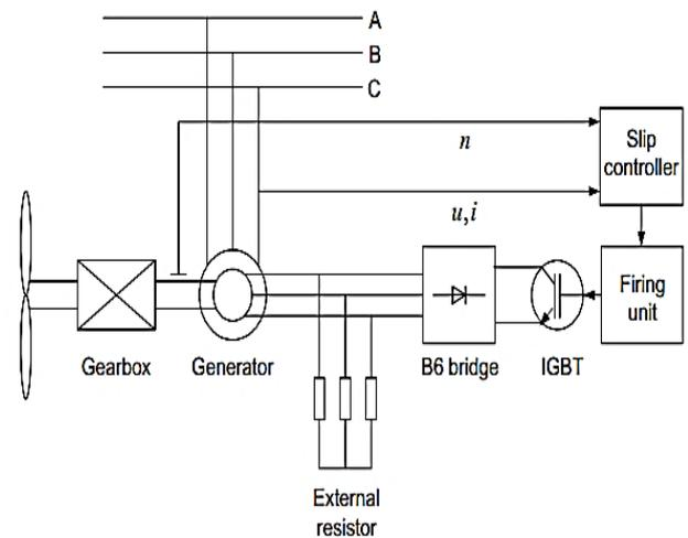
Fig. 2. Dynamic slip control of wind turbine by three-phase external resistor with direct current pulsing.
