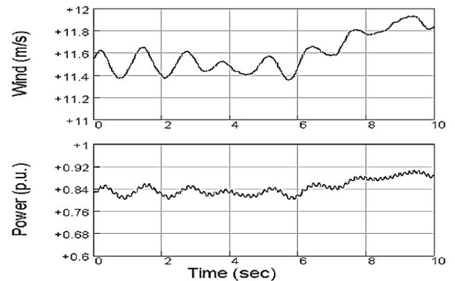
Fig. 5. Wind and output power of the wind turbine in the case of normal operation.
