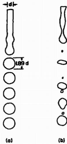
Fig. 7: a) idealized primary breakup b) real primary breakup with satellite droplet formation [26]
