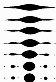
Fig. 3: Evolution of Ligament Stretching and Particle Formation with Satellite Particles [6]
