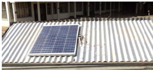
Fig. 3: Experimental setup: PV module attached to CMS and temperature sensors
