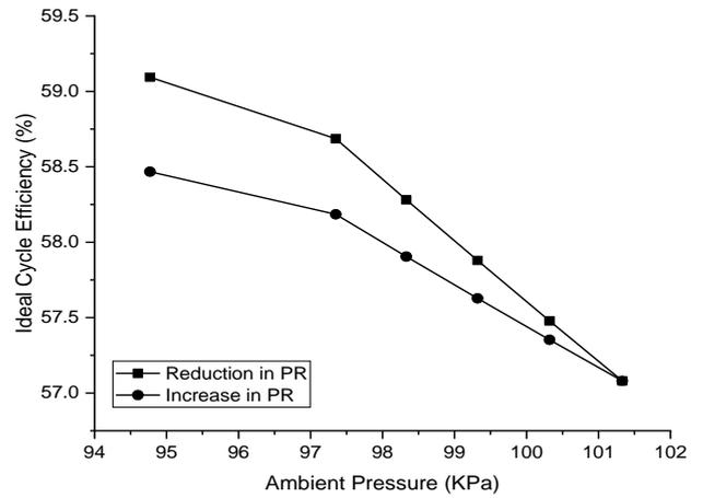
Figure 8: Ideal Cycle Efficiency - Ambient Pressure with HE in Simple Cycle
