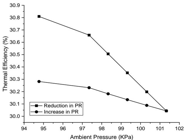
Figure 7: Thermal Efficiency - Ambient Pressure with HE in Simple Cycle
