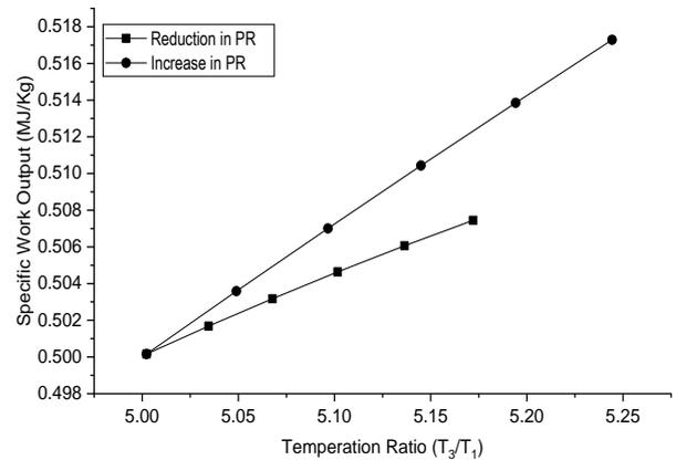
Figure 9: Specific Work Output and Temperature Ratio in a Simple Cycle with HE
