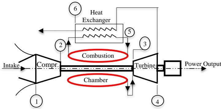
Figure 2: Single Shaft Open Cycle GT with HE
