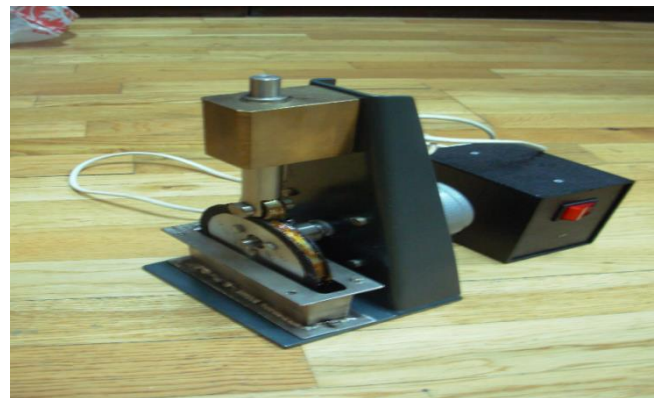
Figure 6. Design version how to save lubricant constantly between zone of contact cam-disc
