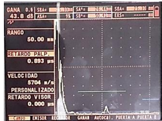
Fig. 1. Screen of the ultrasonic instrument showing the signal waves obtained in CZ zone of the slab sample.
