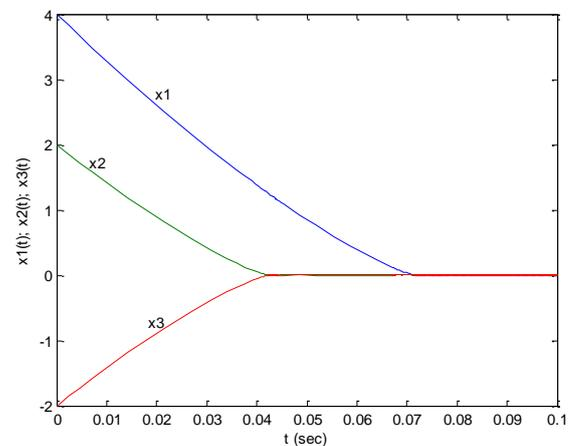
Figure 2: Typical state trajectories of the feedback-controlled system of (1) with (10) and (11).
