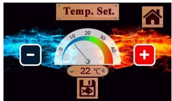
Fig. 11. Touchscreen temperature setting page
