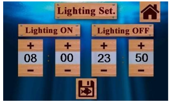
Fig. 16. Touchscreen lighting range setting page
