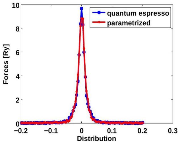
**FIG 1: Forces against distribution in force matching minimization between quantum espresso and parameterized potential**
