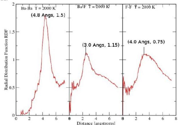
**FIG 7: Radial distribution functions at 2000 K.**
