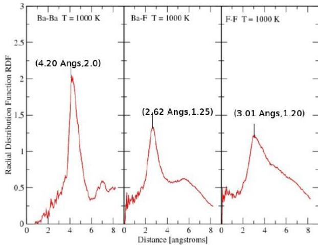
**FIG 4: The radial distributions function at 1000K. Cations and anions are still at their mean lattice positions.**
