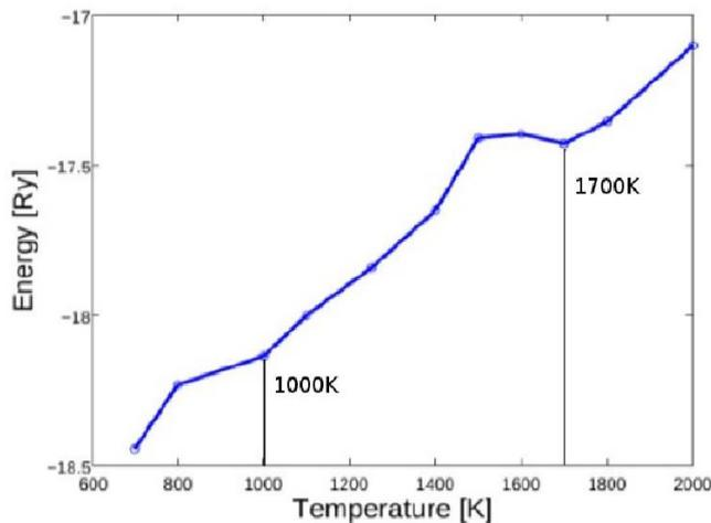
**FIG 2: The temperature dependence of the total energy for the c-BaF<sub>2</sub>**
