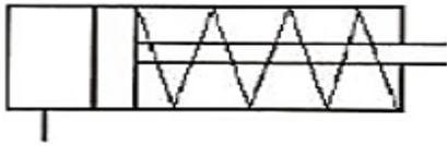
Fig. 3. Cylinder of simple energy with spring return [5]
