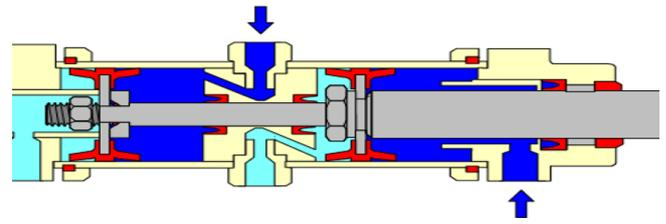
Fig. 8. Double Tandem roller cross section [10]
