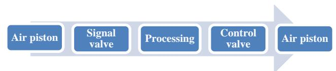
Fig. 1. Logical diagram of a pneumatic system [10]
