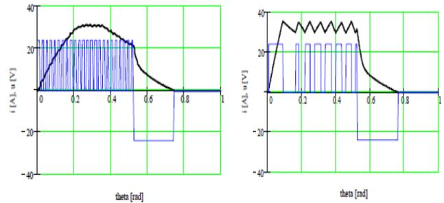
Fig.8. Phase current and voltage as a function of the rotor position, for:
