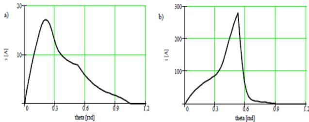
Fig.6. Currents vs. the rotor position at turn-on angle  $\vartheta_{on} = 0$  deg; turn-off angle  $\vartheta_{off} = 30$  deg and speed: a)  $n=4000$  rpm, b)  $n=1000$  rpm.
