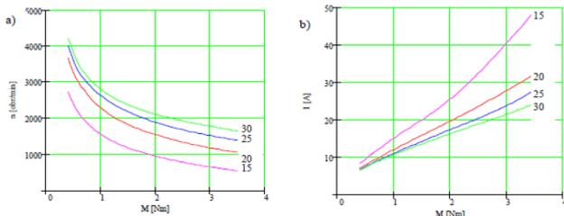
Fig.7. Characteristics at turn-off angle within  $\vartheta_{off} = 15 \div 30$  deg, turn-on angle  $\vartheta_{on} = 0$
