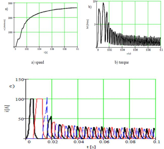
Fig.5. Time waveforms: a) speed; b) torque; c) phase currents during the motor starting For  $M=1.5$  Nm
