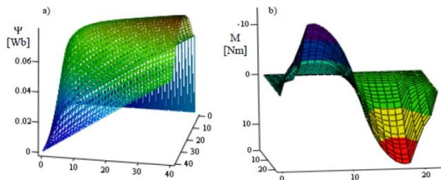
Fig.4. Flux-linkage (a) and static torque, (b) as a function of current and rotor position.
