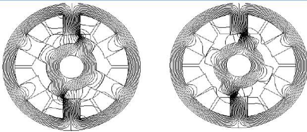
Fig.3. Vector potential distribution when supplying one of the phase winding  $I=10$  A for different
