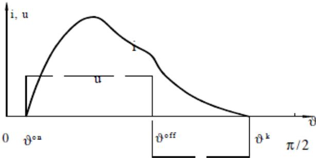
Fig.2. Phase current and voltage vs. rotor position.
