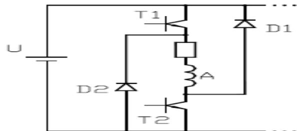
Fig.1. Controller circuit for one motor phase.
