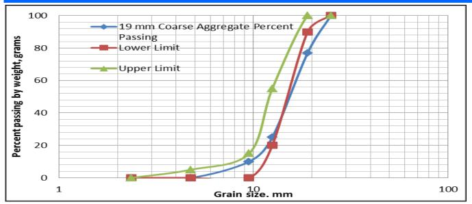
Figure 2: The coarse aggregate 19 mm granite grain size distribution curve
