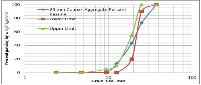
Figure 3: The coarse aggregate 25 mm granite grain size distribution curve
