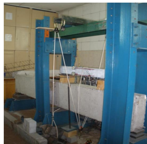
Figure-2: Overview of test setup for long-term loading
