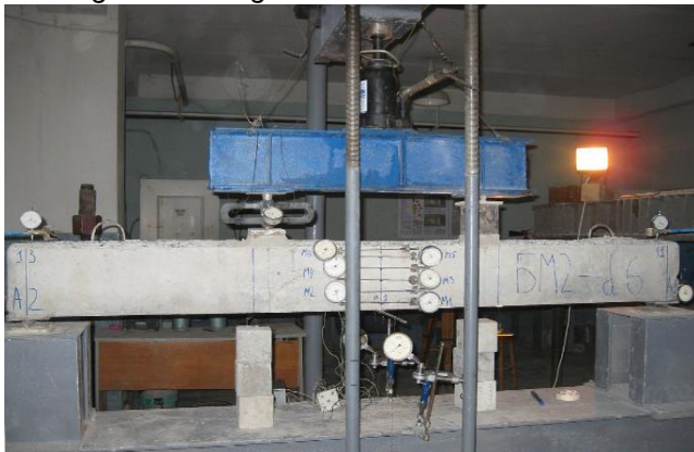
bending structures reinforced with composite armature
