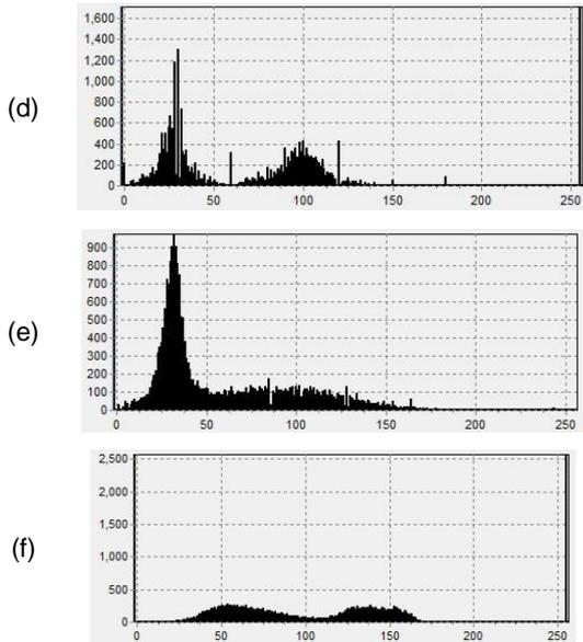
Fig. 4. Histogram for H, S and V component applied to road 2 a). d) H Histogram (a). e) S Histogram (b) and, f) V Histogram(c).
