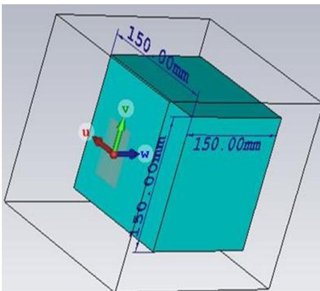
Fig.3. Geometry model of the proposed antenna with the tissue.
