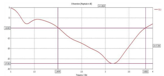
Fig.4. The return loss at less than -10dB with impedance bandwidth of 2.0228GHz – 3.8441GHz.
