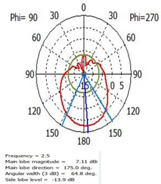
Fig.5. Far field of 7.11 dB at the centre frequency of 2.5 GHz.
