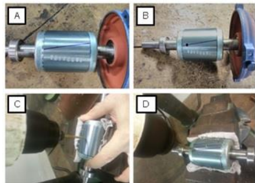
Fig. 3. Rotors: a) healthy; b) one broken bar; c) two broken bars, and d) three broken bars.
