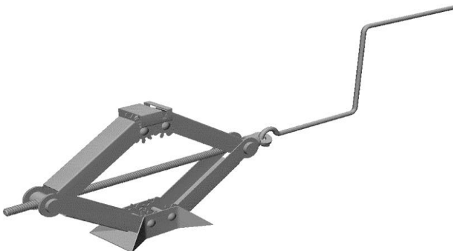
Fig. 2. Model drawing for the scissor jack.
