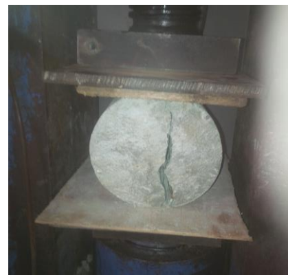
Figure 4 Tensile splitting strength test
