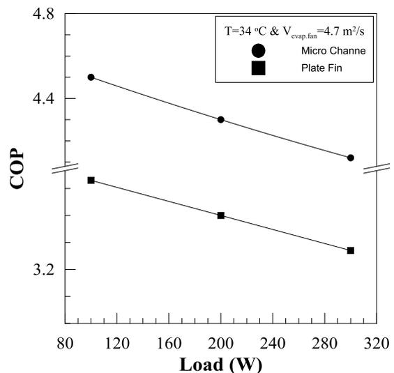
Fig. (9) coefficient of Performance vs. load imposed on evaporator
