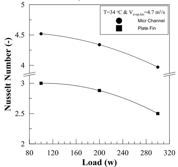
Fig. (5) Nusselt Number vs. load imposed on evaporator
