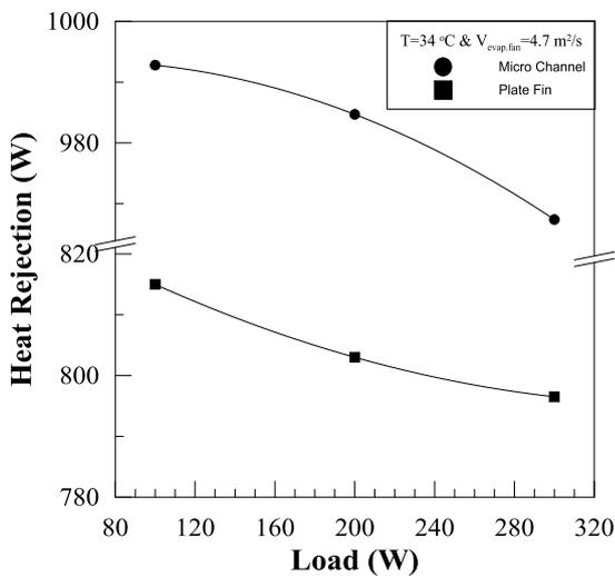
Fig. (7) heat rejection vs. load imposed on evaporator
