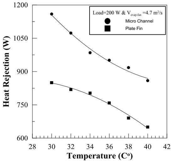
Fig. (6) heat rejection vs. ambient temperature
