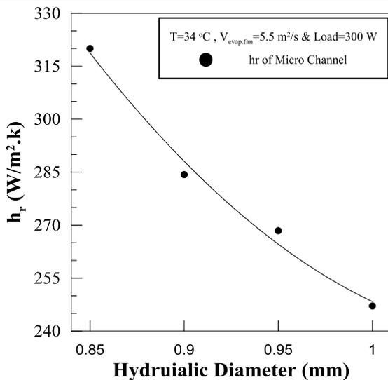
Fig. (10) variation of heat transfer coefficient vs. channel hydraulic diameter
