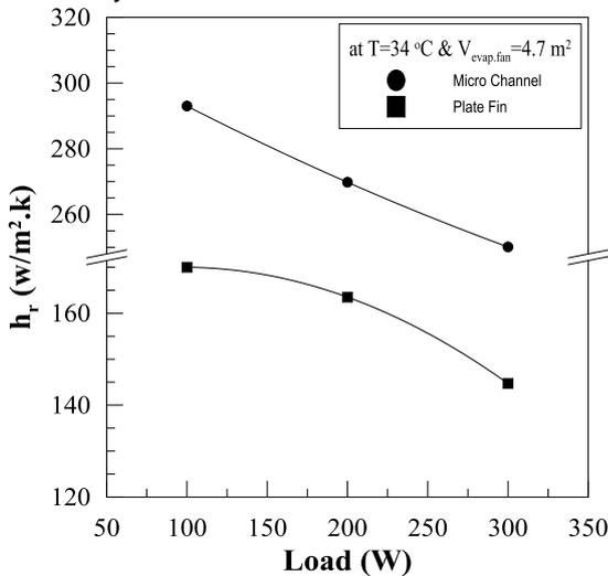
Fig. (3) theoretical heat transfer coefficient vs. load imposed on evaporator.
