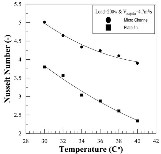
Fig. (4) Nusselt number vs. ambient temperature
