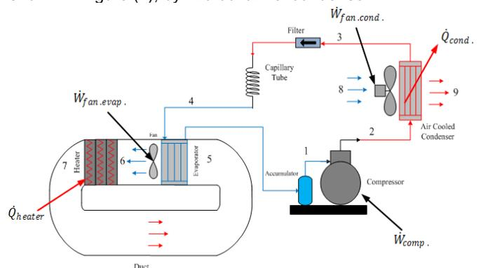
Fig. (1) Schematic Diagram of the Vapor compression cycle
