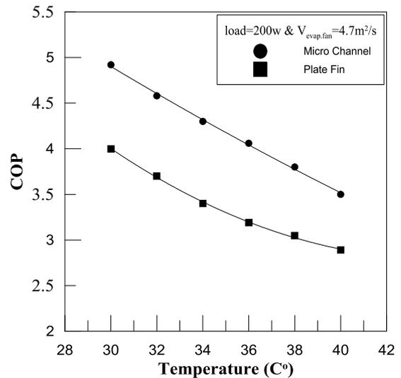
Fig. (8) coefficient of Performance vs. ambient temperature
