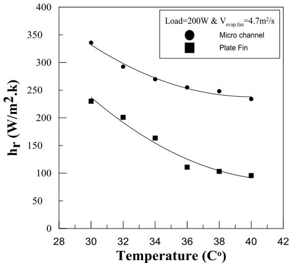
Fig (2) theoretical heat transfer coefficient vs. ambient temperature
