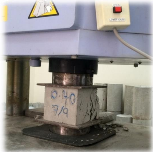
Fig.7 Destructive testing for cubes
